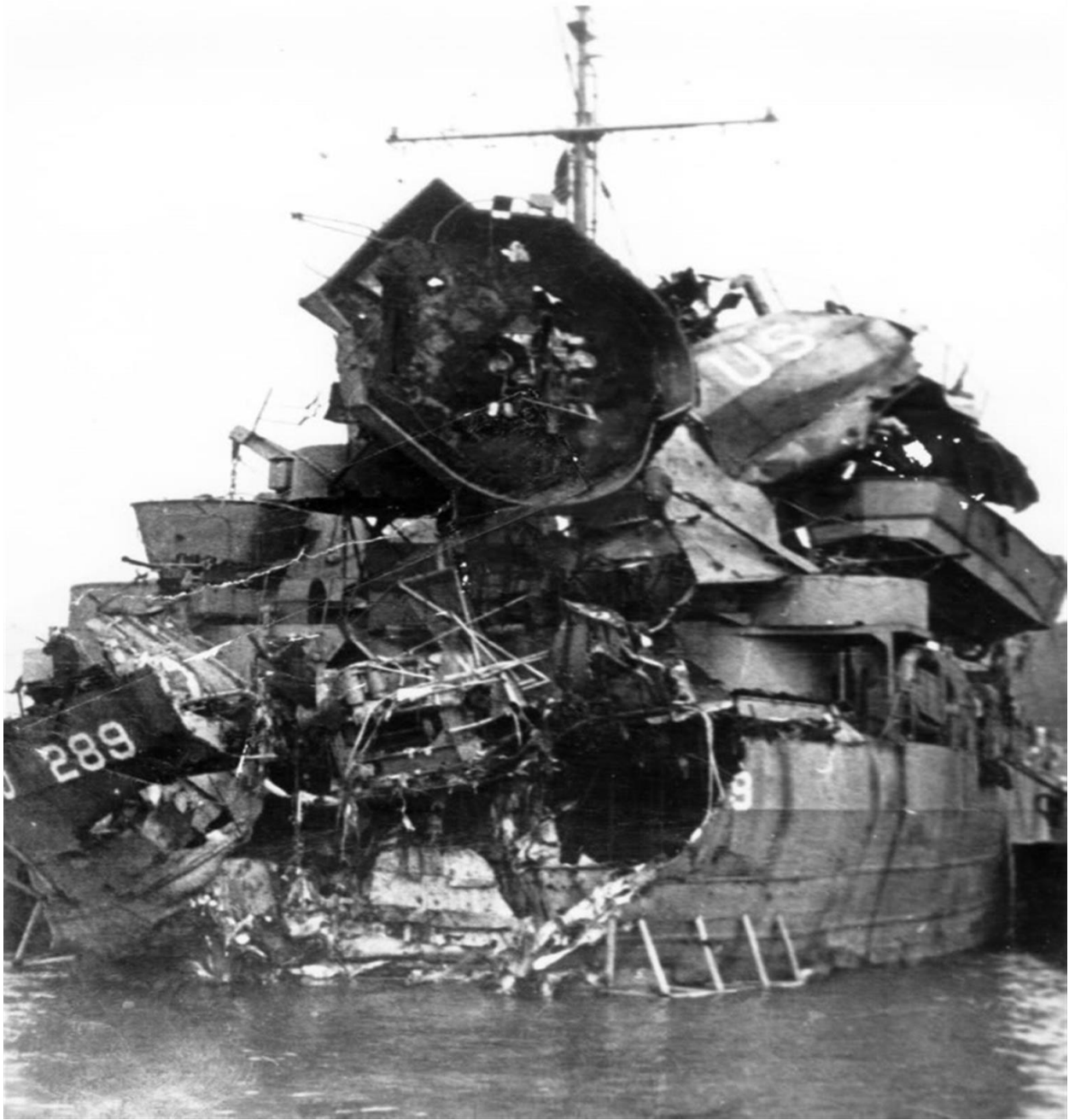
LST 289 at Dartmouth Harbor, England torpedo damage. Photograph by US Navy.
