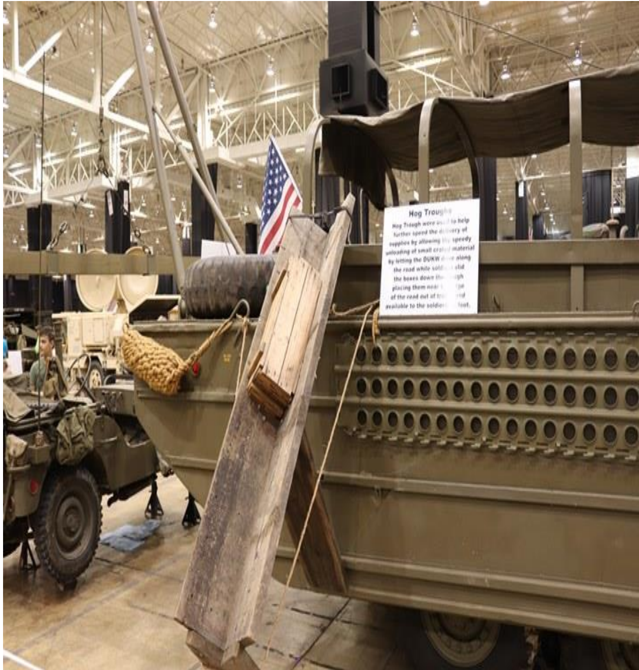
DUKW aka Duck a “hog trough”, a simple two-piece lumber with legs assembled to unload cases of ammunition, food, and petroleum much faster at predetermined dump sites.
